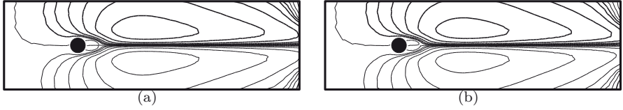
Figure 14. Empirical (left) and a priori (right) shift mode. The empirical mode is computed from the mean flow and steady solution as described in (Noack et al., 2003). The a priori shift mode is derived from the Reynolds equation using the POD representation of the Reynolds stress tensor.
